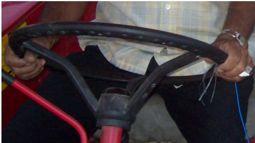
Fig 1: Mounting of accelerometer and hand adapter on handle of the hand tractor
