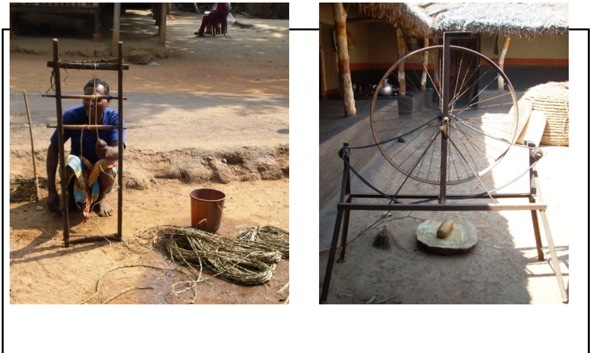
Photograph 4: Traditional Gurru (Rope twisting hand operated devices)
