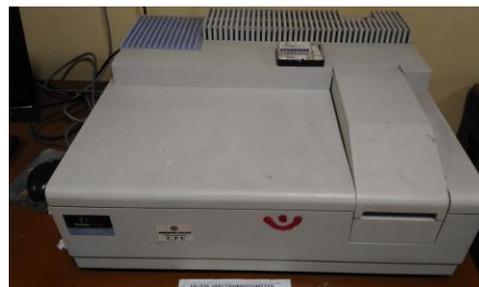
**Fig. 2.7.** Schematic set-up of Lambda-35 double beam UV/Vis spectrophotometer.
