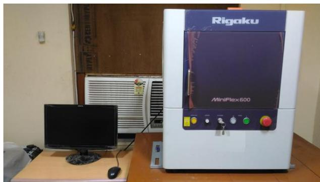
**Fig. 2.3.** Representation of XRD experimental set-up.
