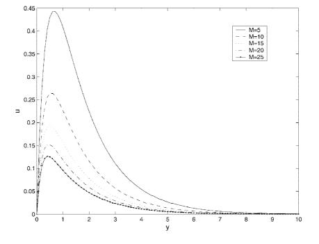
Fig.1 Main flow velocity u for Gr = 5.0, S = 1.0, Pr = 0.72, z = 0.0,  $\in$  = 0.2
