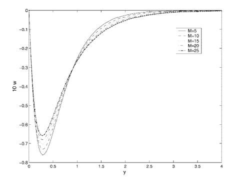
Fig.2 Cross velocity  $10 \times w$  for S = 1.0, Pr = 0.72, z = 0.5,  $\in = 0.2$
