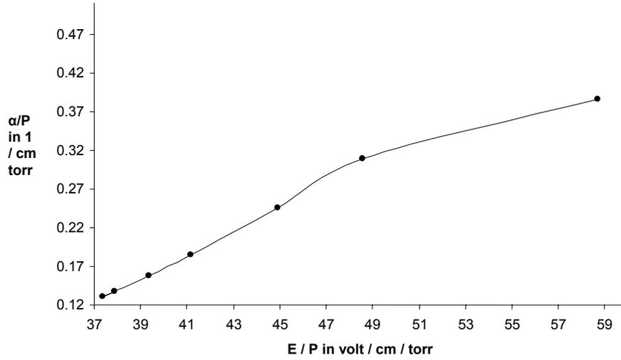
**Figure 3:** Variation of  $\alpha/P$  with  $E/P$  for Torus A with Hydrogen gas
