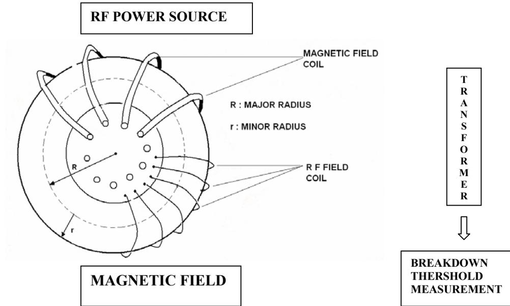
Figure :1 The Schematic Diagram Of The Experimental Set Up
