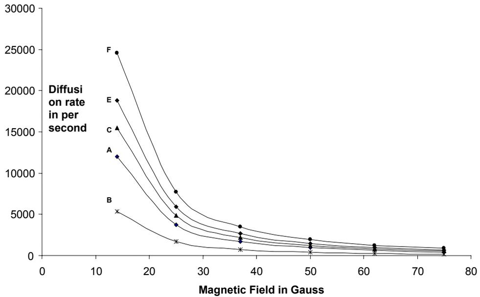
FIGURE 5: Variation of diffusion loss rate with magnetic field in different torii .
