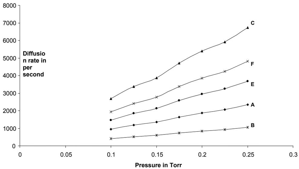
FIGURE 6 : Variation of diffusion loss rate with pressure at a constant magnetic field of 50 gauss in different torii.
