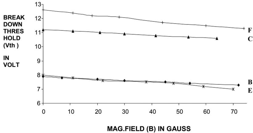
**FIGURE 2:** Variation of breakdown threshold voltage with magnetic field at a constant pressure of 0.1 torr for different torii with pre ionisation condition for hydrogen
