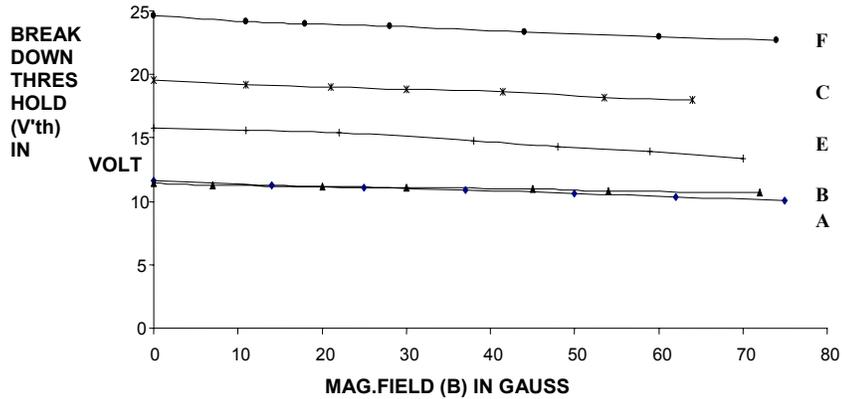
**FIGURE 3:** Variation of breakdown threshold voltage with magnetic field at a constant pressure of 0.1 torr for different torii without pre ionisation condition for hydrogen
