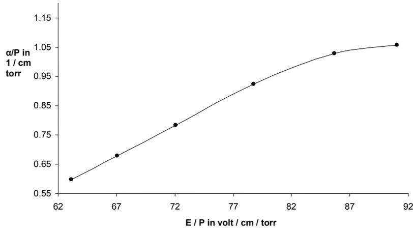
**Figure 4:** Variation of  $\alpha/P$  with  $E/P$  for Torus C with Hydrogen gas
